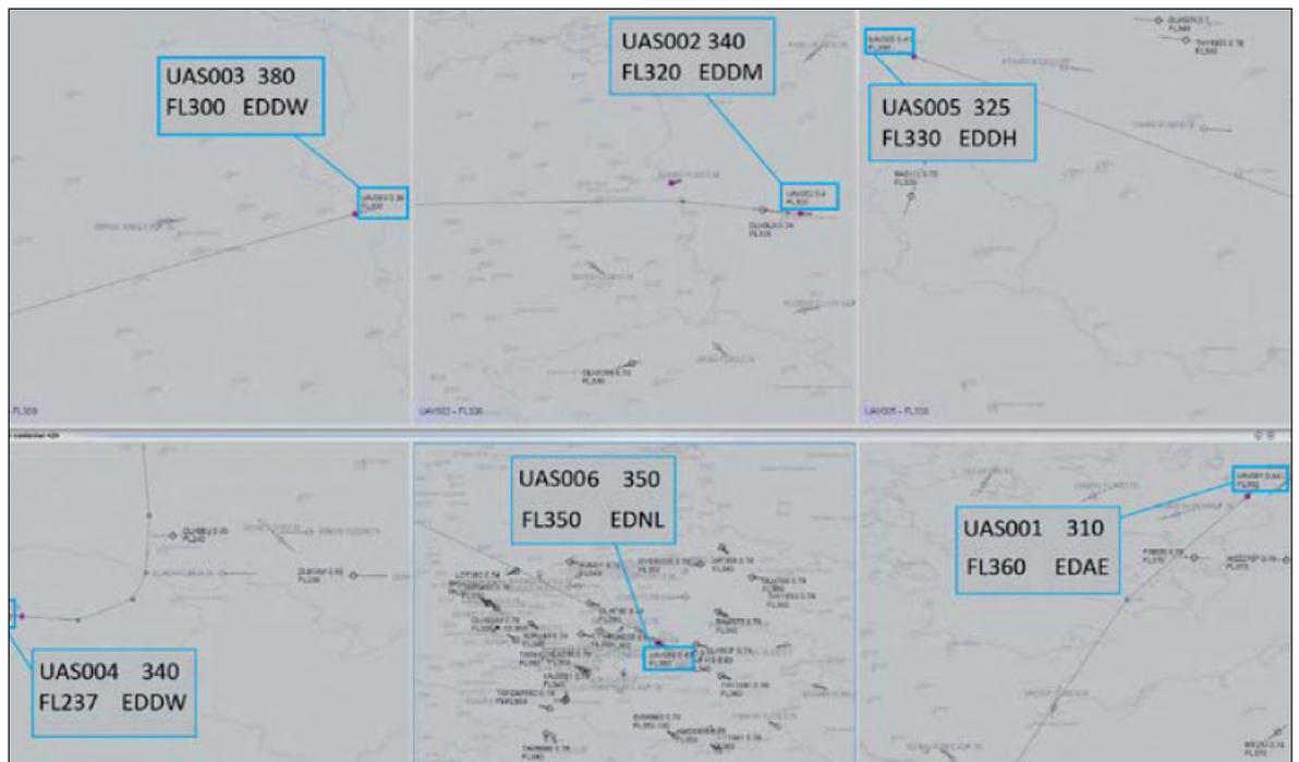
Figure. 2: ATC display for UA control. Conceptual display for an UA controller with responsibility to control and monitor 6 UAS simultaneously in a sector-less airspace.
